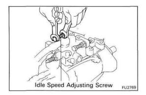
(d) Adjust by turning the idle speed adjusting screw.
